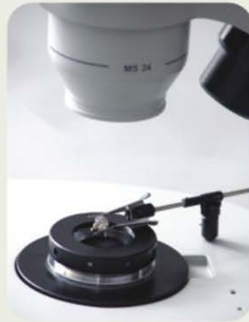
Gems - Inspection Accessories Darkfield attachment (with specimen holder) for inspection of Gems & Micro samples under transmitted light
